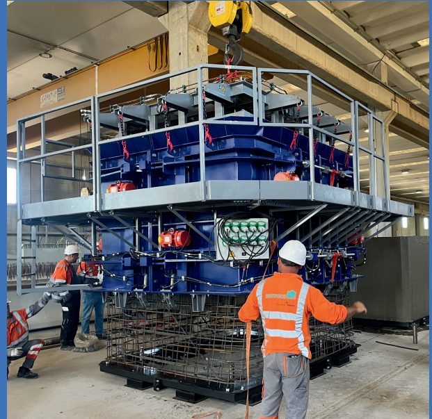
MOULDS FOR BOX CULVERTS
