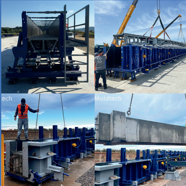
MOULDS FOR COLUMNS
