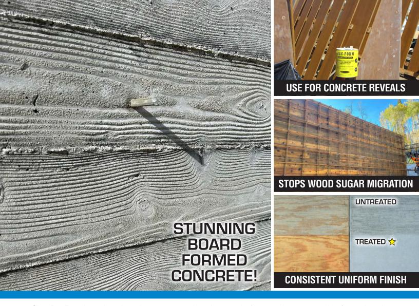
Clear Pre-Form is a solvent based, transparent, polyurethane sealer for protecting most wood surfaces. It works by reducing water absorption into the wood, thus minimizing the migration of dissolved wood sugars and tannins into the concrete. Resulting concrete surfaces are typically uniform in color and free of dusting caused by wood sugar retardation.
